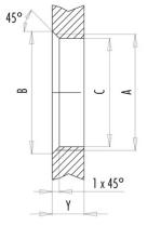
Installation direction: o-ring sits on chamfer.
